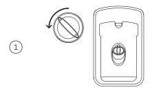
Turn the cap anticlockwise and remove.
